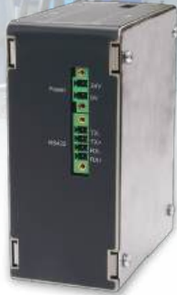
RIO16 DIN rail mount Digital I/O unit
