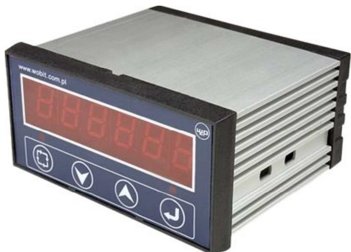
MD150T is universal processing display designed to measure signals from load cells and force sensors. Built-in analogue-to-digital converter allows for measurement with resolution up to 100 000 of measuring range. The result is presented on six position display. MD150T has multipurpose usage as well at industry as in laboratory. Depends on used sensor there is a possibility of measurement as well small forces as large. Measured data can be downloaded to PC.
