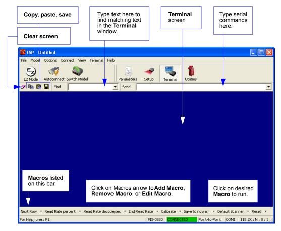
The **Terminal** interface allows the user to send serial commands to the scanner by using macros, by copying and pasting, or by typing commands in the **Send** text field.
