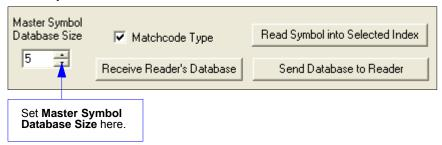
**Important:** Since the total number of characters available for the master symbol database is **3000**, changes to the **Master Symbol Database Size** will re-allocate the number of characters available for each master symbol and could cause existing master symbols to be deleted (except master symbol #1, unless it also exceeds the size limitation).
