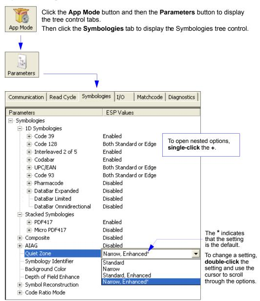
**Note:** Symbologies settings can also be sent to the scanner from ESP's Terminal using wenglor's K command format. Refer to the **Symbologies** section of **Appendix C**.
