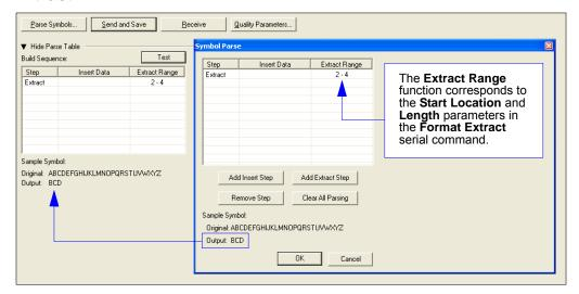
Multiple character sequences can be extracted and inserted using **Symbol Parse**. In this example, the selected extraction range is characters 2-4. The "Sample Symbol" example on the **Symbol Parse** dialog shows the selected character positions extracted and output as desired. Simultaneously, the data string from the selected symbol is displayed at the bottom left of the **Parse Table**, followed by the user-defined extracted output.
