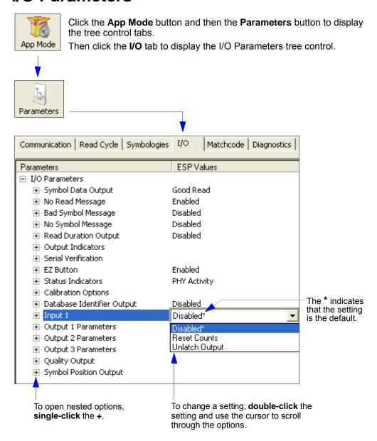
**Note:** I/O Parameters settings can also be sent to the scanner from ESP's Terminal using wenglor's K command format. Refer to the I/O Parameters section of Appendix C.
