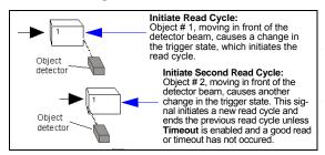
This mode is highly recommended in any application where conveying speed is constant, or if spacing, object size, or read cycle timeouts are consistent.
