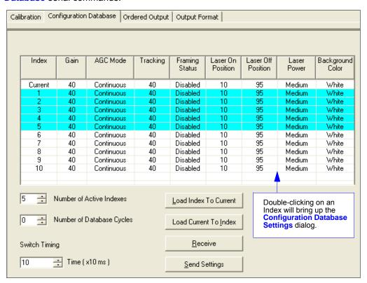
Use the Number of Active Indexes field to determine how many database indexes will be used. Use the Number of Database Cycles to determine how many times the active indexes will be repeated. Use the Switch Timing field to determine the amount of time between active indexes.
