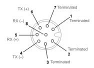
Important: The 8-pin Ethernet version of Connector B does not have RS-422/485, Input 1, or RTS/CTS pins.
