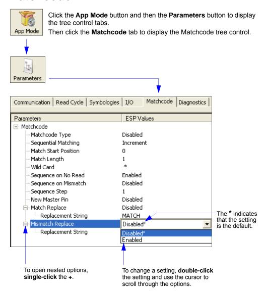
**Note:** Matchcode settings can also be sent to the scanner from ESP's Terminal using wenglor's K command format. Refer to the **Matchcode** section of **Appendix C**.
