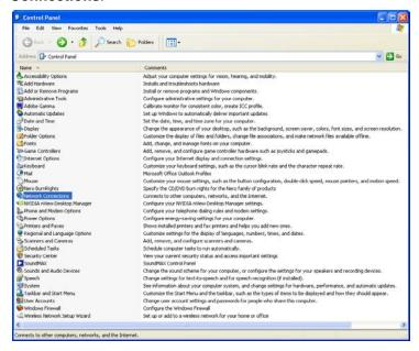
2. The **Network Connections** dialog will appear. Double-click the icon for the Local Area Connection being used in the application.
