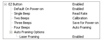
The EZ Button has four positions: **Single Beep**, **Two Beeps**, **Three Beeps**, and **Four Beeps**, selectable by the length of time the button is held down, and indicated by one, two, three, and four beeps in succession. Each position can be programmed for any of eight **EZ Button Modes**.
