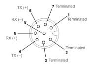
Connector B (Ethernet) M12 8-pin Socket
