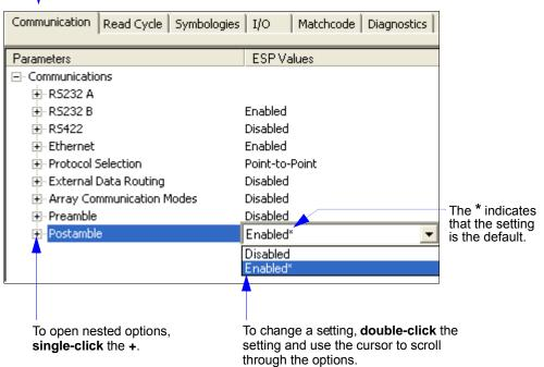
**Note:** Communication settings can also be sent to the scanner from ESP's Terminal using wenglor's K command format. Refer to the **Communication** section of **Appendix C**.
