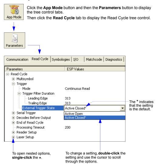
**Note:** Read Cycle settings can also be sent to the scanner from ESP's Terminal using wenglor's K command format. Refer to the **Read Cycle** section of **Appendix C**.
