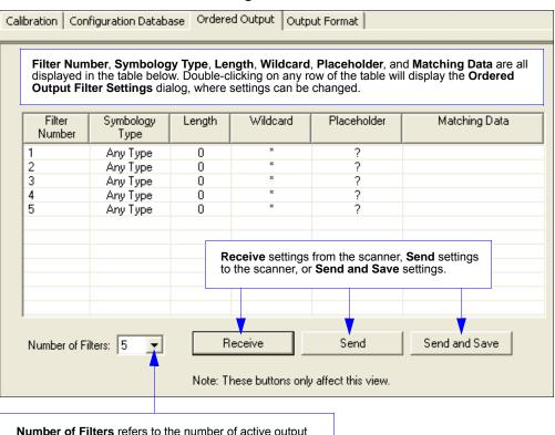
**Number of Filters** refers to the number of active output filters. **0** disables all output filters. Any non-zero numeral will enable output filtering to be performed using the filter indexes covered by this value.
