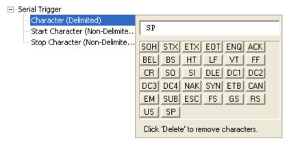
**Note: Serial Data** or **Serial Data and Edge** trigger mode must be enabled for **Serial Trigger Character** to function.
