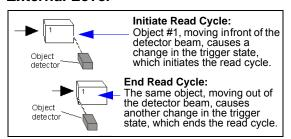
This mode is effective in an application where the speeds of the conveying apparatus are variable and the time the scanner spends reading each object is not predictable. It also allows the user to determine if a No Read has occurred.
