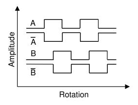
Output Signals TTL (3 Channels) Sense of Rotation: CW (Clockwise)
