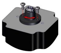
Recommendation for mounting screws: 4-40 1/4" Max. allowed tightening torque 0.67 Nm.
